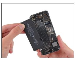
Pull the battery out of the rear case.
