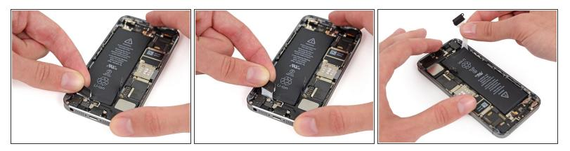
• Pull the outside battery adhesive tab straight up and carefully around the corner of the battery.
