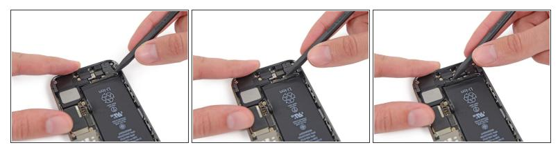
Run the tip of a spudger between the battery and the headphone jack to unfold the battery adhesive tab.
