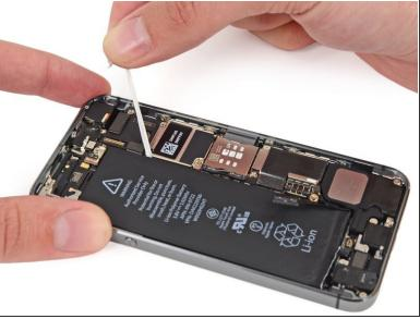
Pull the strip along the side of the battery until the strip comes free from the phone.
