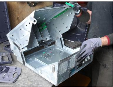
After removing the motherboard, the casing should be completely blank.
