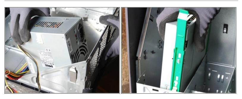
Once all wires and cables have been disconnected the drives (floppy drive, CD drive and hard disk drive, etc.) can be removed. Also remove the power supply.
