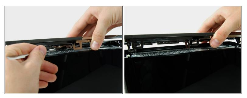
(i) This clip is smaller than the others and should not be removed from above like the others.
