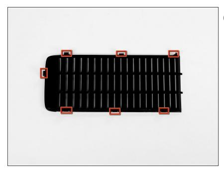
(i) In the following steps, you will remove the bottom vent. It is attached to the bottom panel by the seven clips shown.
