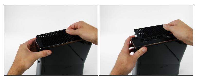
• Remove the bottom vent by lifting it away from the bottom bezel.
