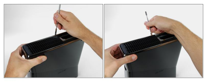
(i) Orient the Xbox 360 S so that the hard drive port is facing up and the faceplate is facing to the left.
