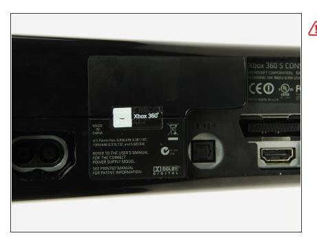
Opening your Xbox 360 any further will require breaking or removing the warranty sticker on the outer case. Your Microsoft warranty for any components not directly attached to the logic board will likely be voided by removing this seal.
