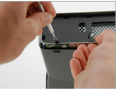
Using the same method described above, free the two remaining clips along the left edge of the top bezel.
