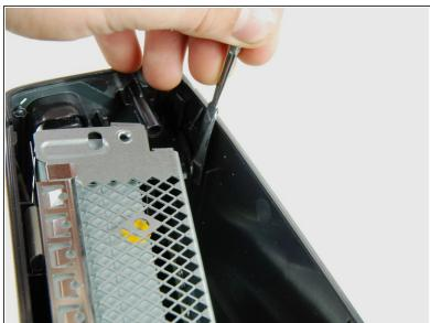
• Release one clip in the front left corner of the top edge securing the left case to the faceplate.
