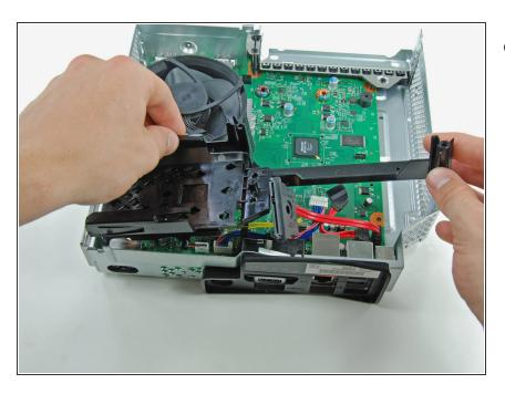
Lift the hard drive bracket out of the metal frame.
