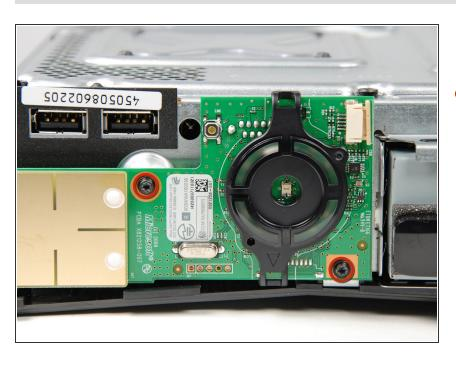
Remove the two 5.6 mm T8 Torx screws securing the RF module to the metal case.
