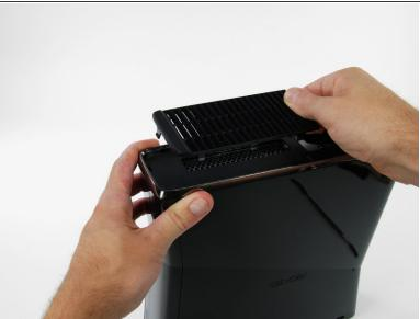
Remove the bottom vent by lifting it away from the bottom bezel.
