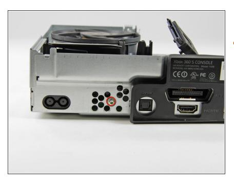
Remove the 11.3 mm T10 Torx screw holding the hard drive bracket to the metal frame, near the DC-In port.
