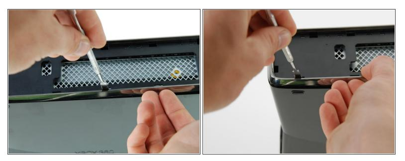
Using the same method described above, free the two remaining clips along the left edge of the top bezel.
