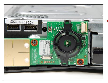
Remove the two 5.6 mm T8 Torx screws securing the RF module to the metal case.
