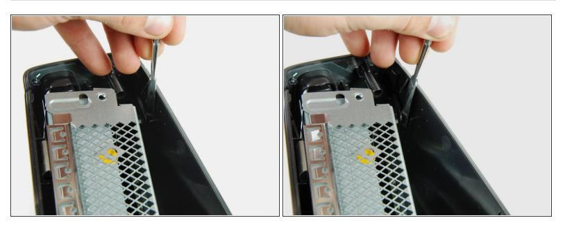
• Release one clip in the front left corner of the top edge securing the left case to the faceplate.
