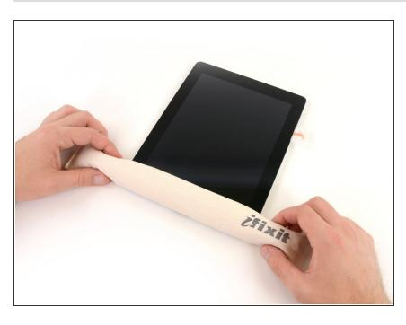
While you work on releasing the adhesive on the right side of the iPad, reheat the iOpener, and replace it on the bottom edge of the iPad.
