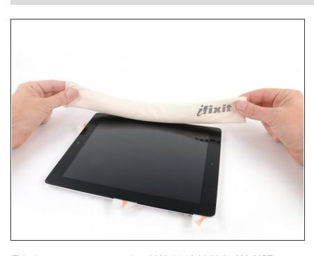
Reheat the iOpener in the microwave and set it on the left edge of the iPad to start warming the adhesive in that section.
