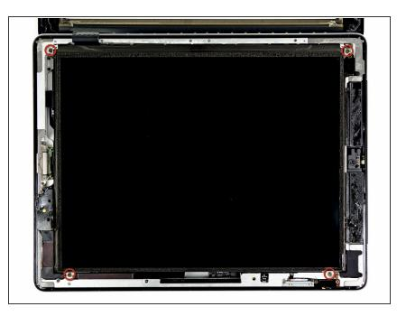
Remove the four 2.0 mm Phillips #0 screws securing the LCD to the rear case.
