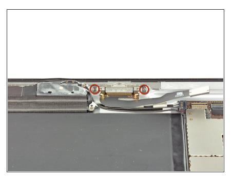
Remove the two 2.0 mm Phillips screws securing the dock connector to the rear panel.
