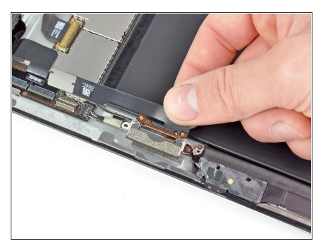
Pull the dock connector away from the edge of the rear panel and remove it from the iPad 2.
