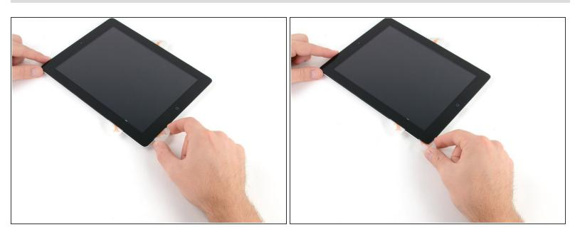
Using the opening pick that is still underneath the bottom edge of the iPad, release the adhesive along the bottom left corner.
