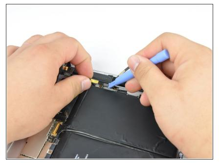
• Use the edge of a plastic opening tool to disconnect the microphone cable connector.
