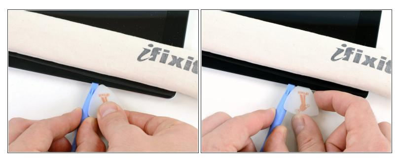
• Keeping the tip of the plastic opening tool wedged between the front glass and plastic bezel, slide a plastic opening pick in the gap, right next to the plastic opening tool.
