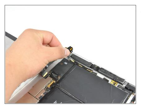
• Carefully peel the front camera and microphone cables off the rear panel.
