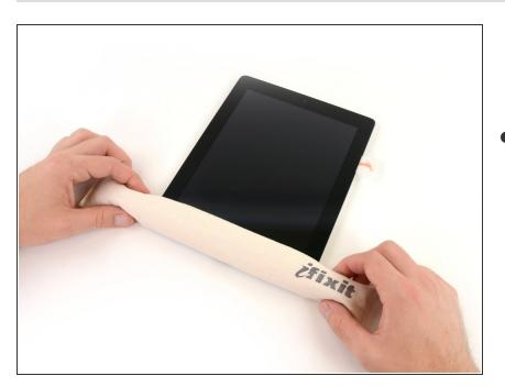
While you work on releasing the adhesive on the right side of the iPad, reheat the iOpener, and replace it on the bottom edge of the iPad.
