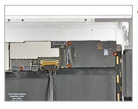
Remove the four 2.6 mm Phillips screws securing the logic and communications boards to the rear panel.
