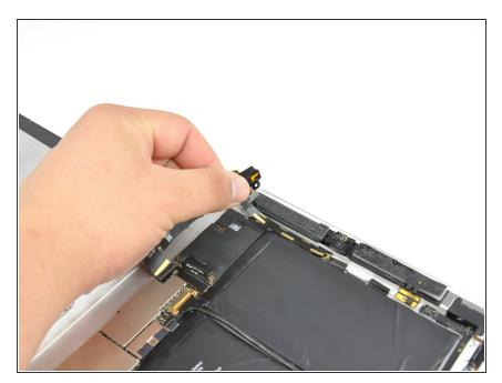
Carefully peel the front camera and microphone cables off the rear panel.
