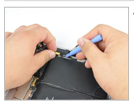
Use the edge of a plastic opening tool to disconnect the microphone cable connector.
