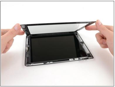
Holding the iPad by the top and bottom right corners, rotate the front glass away from the iPad.
