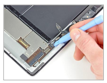
Pry the speaker cable connector straight up from its socket on the logic board.
