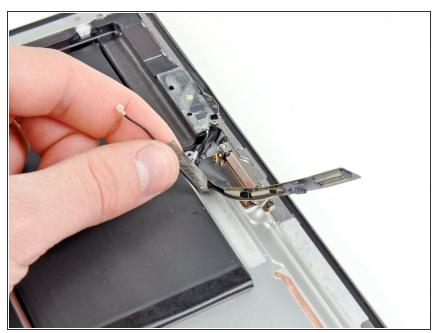
Move the dock connector/speaker cables out of the way and peel the bluetooth/wi-fi antenna cable off the adhesive securing it to the rear case.
