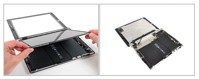
• The front panel ribbon cables are connected beneath the LCD. To access them, you'll need to temporarily flip the LCD over and out of the way.
