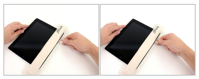
Remove the plastic opening tool from the iPad, and push the opening pick further underneath the front glass to a depth of ~0.5 inches.
