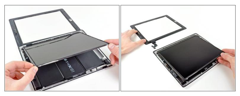
(i) In order to remove the front panel assembly, the ribbon cable needs to slide out between the case and the LCD. You'll need to move the LCD to make some room.
