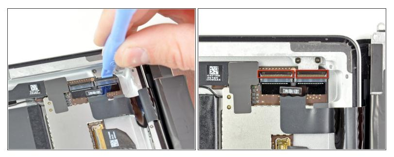
• Use the edge of a plastic opening tool to carefully flip up the retaining flaps on the two digitizer ribbon cable ZIF sockets.
