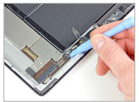
Pry the speaker cable connector straight up from its socket on the logic board.
