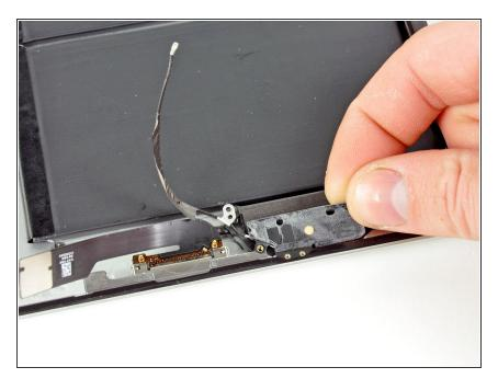
Peel the bluetooth/wi-fi antenna off the speaker enclosure and remove it from the iPad 2.
