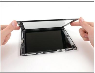
Holding the iPad by the top and bottom right corners, rotate the front glass away from the iPad.
