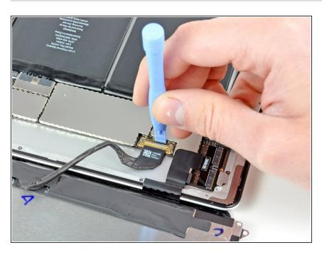
Use the edge of a plastic opening tool to flip up the metal retaining clip securing the display data cable to its socket on the logic board.
