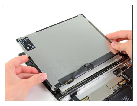
Remove the LCD assembly from the iPad 2.
