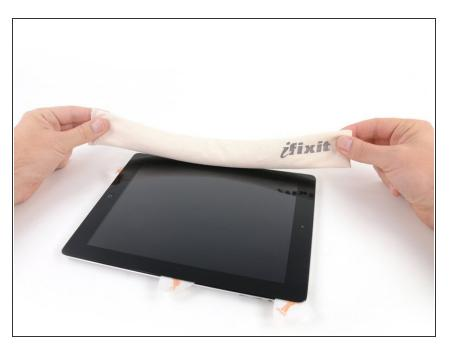
Reheat the iOpener in the microwave and set it on the left edge of the iPad to start warming the adhesive in that section.
