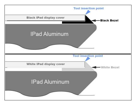
Make sure you place the tool in the proper spot—between the plastic display bezel and the front panel glass.
