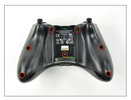
Remove the seven 9.3 mm T8 Security Torx screws securing the rear case to the front case.
