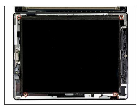
Remove the four 2.0 mm Phillips screws securing the LCD to the rear case.
