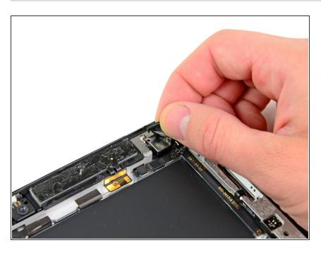
Carefully peel the rubber cover off the metal camera retainer and remove it from the iPad 2.
