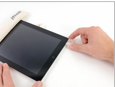
Slide the opening pick around the bottom right corner of the iPad, releasing the adhesive there.
