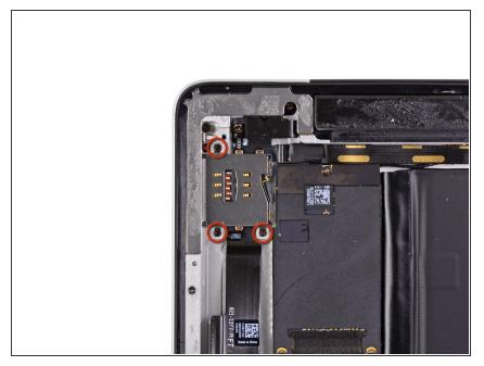
Remove the three 2 mm Phillips screws securing the SIM card slot to the rear panel.
