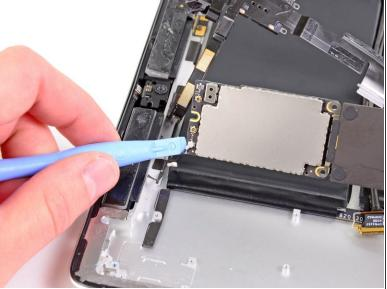
Use a plastic opening tool to disconnect both antenna connectors from their sockets on the communications board.
