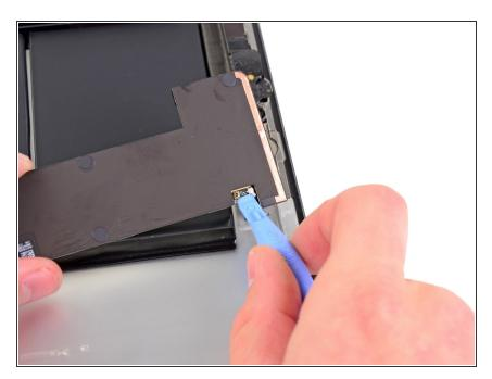
Disconnect the Wi-Fi antenna connector from its socket on the logic board.
