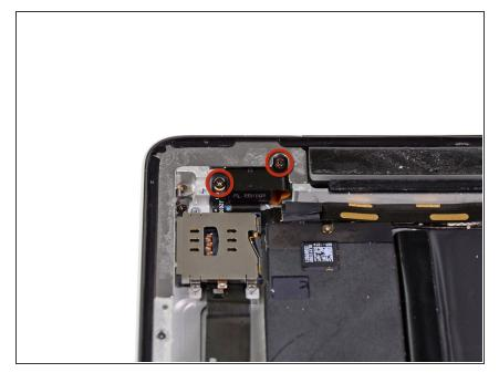
Remove the two 2.9 mm Phillips screws securing the headphone jack to the top edge of the rear panel.
