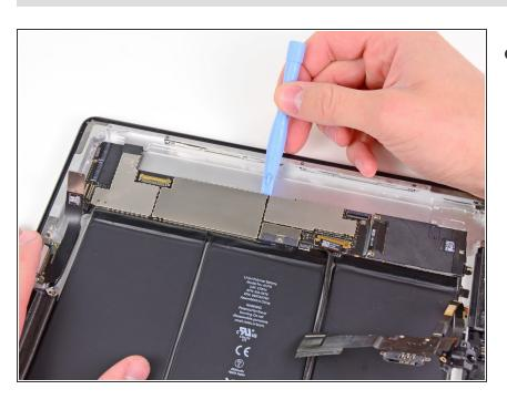
Use the edge of a plastic opening tool to gently pry the logic board up from the adhesive securing it to the rear case.
