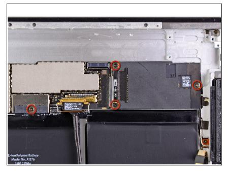
Remove the four 2.6 mm Phillips screws securing the logic and communications boards to the rear panel.
