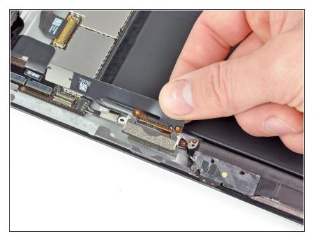
• Pull the dock connector out of its slot in the rear case and remove it from the iPad 2.
