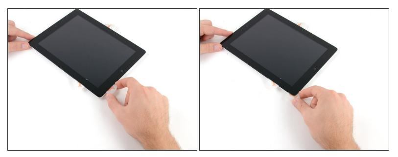
• Using the opening pick that is still underneath the bottom edge of the iPad, release the adhesive along the bottom left corner.
