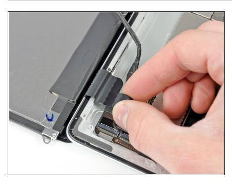
Pull the digitizer ribbon cable straight out of its two sockets on the logic board.
