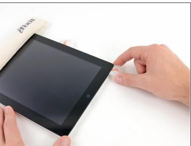
Slide the opening pick around the bottom right corner of the iPad, releasing the adhesive there.
