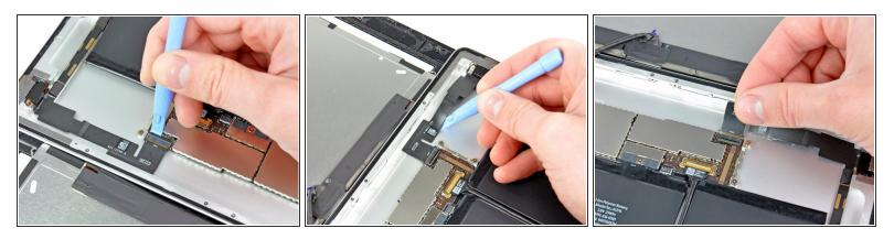
• Use the flat end of a plastic opening tool to flip up the retaining flap on the headphone jack and front-facing camera ribbon cable ZIF socket.
