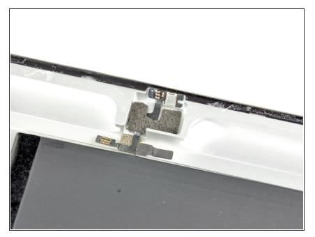
• Peel the piece of foam up off the top of the microphone cable assembly.
