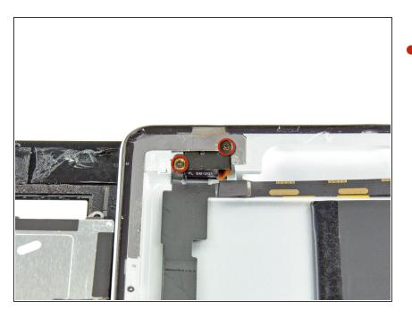
Remove the two 2.9 mm Phillips screws securing the headphone jack to the rear panel.
