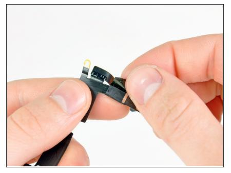
• Carefully remove the strip of tape covering the front camera cable connector.
