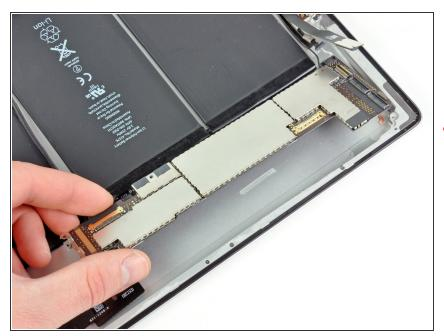
• Lift the logic board out from the rear case and tilt it slightly toward the battery.
