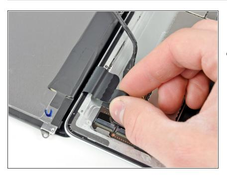
Pull the digitizer ribbon cable straight out of its two sockets on the logic board.
