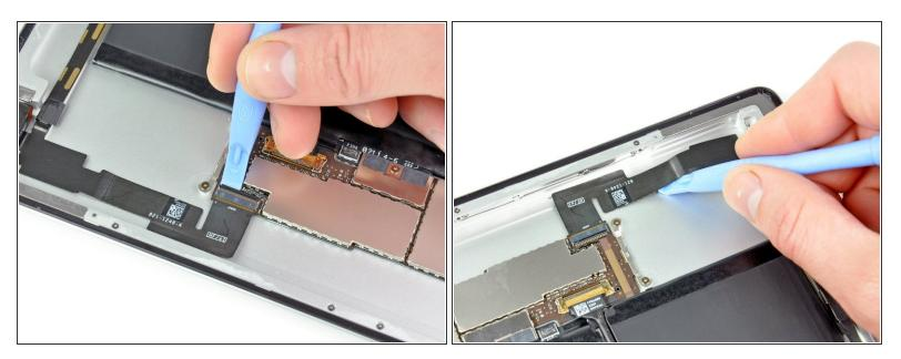
Use the edge of a plastic opening tool to flip up the retaining flap on the headphone jack and front camera cable ZIF socket.
