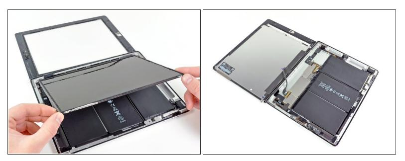
(i) The front panel ribbon cables are connected beneath the LCD. To access them, you'll need to temporarily flip the LCD over and out of the way.
