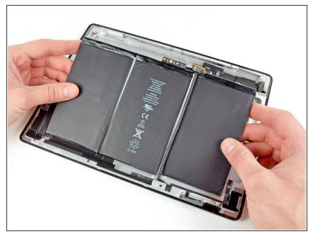
Carefully lift the battery out of the rear panel and remove it from the iPad 2.
