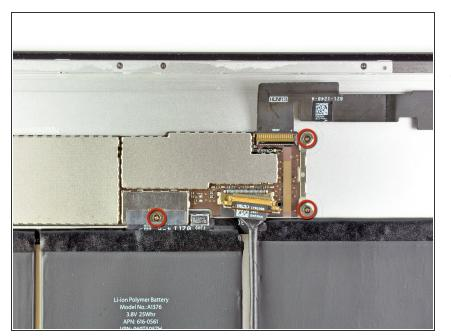
Remove the remaining three 2.6 mm
