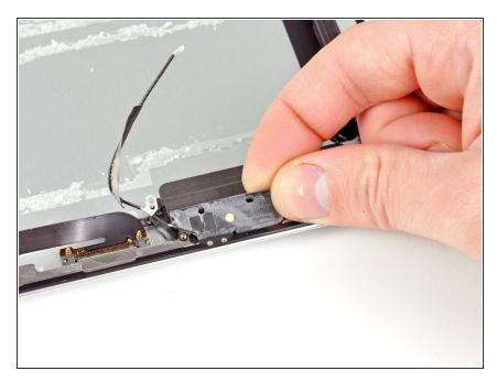
• Peel the Wi-Fi antenna off the speaker enclosure and remove it from the iPad 2.
