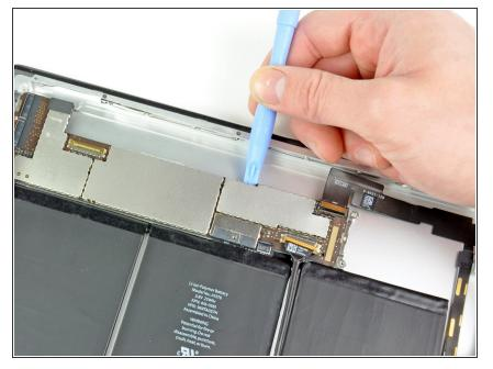
Use the edge of a plastic opening tool to gently pry the logic board up from the adhesive securing it to the rear case.
