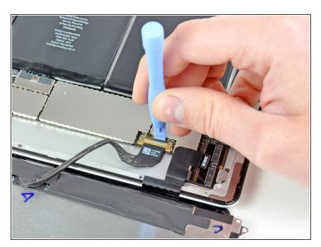
Use the edge of a plastic opening tool to flip up the metal retaining clip securing the display data cable to its socket on the logic board.
