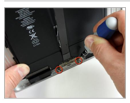
Remove the two 2.84 mm T5 Torx screws securing the dock connector cable to the rear case.
