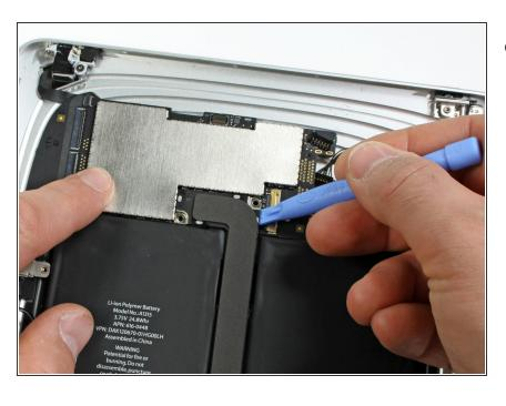
Use the edge of an iPod opening tool to carefully pry the dock cable connector straight up off the logic board.
