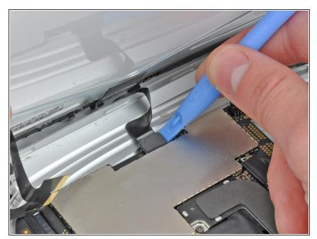
Use an iPod opening tool to remove the ambient light sensor connector from its socket by gently prying upward.
