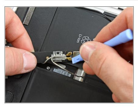
Pry the Wi-Fi and Bluetooth antennas up off their respective sockets on the Wi-Fi/Bluetooth board.
