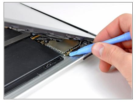
• Use the flat end of a spudger to pry the antenna connector closest to the bottom of the iPad up off its socket on the communications board.
