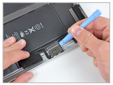
• Use an iPod opening tool to release the SIM board from the adhesive securing it to the rear case.
