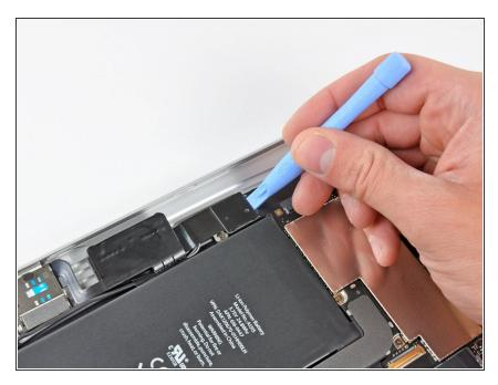
• Use the edge of an iPod opening tool to pry the SIM board connector up off its socket on the logic board.
