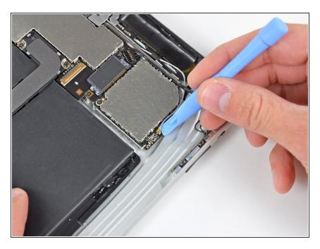
Use the edge of an iPod opening tool to carefully pry the remaining antenna connector up off the communications board.
