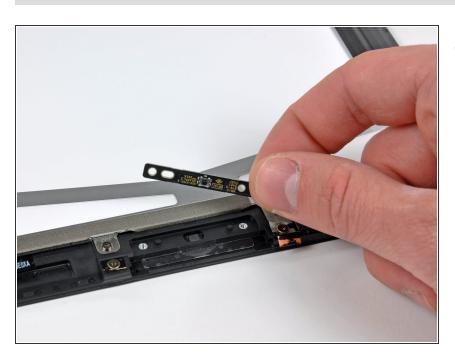
Remove the home button switch board from the display frame.
