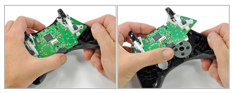
• Lifting from the headphone jack and power plug, remove the logic board from the front case.
