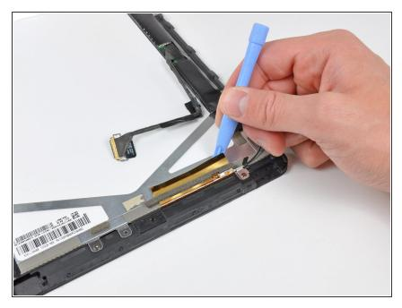
• Use the edge of an iPod opening tool to peel the antenna off the adhesive securing it to the top edge of the display.
