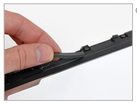
(i) If present, remove the strip of foam tape along the long edge of the display assembly near the digitizer cable.
