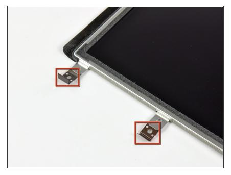
If they are still in good shape, transfer the clips and EMI tape near the bottom of the LCD to your new LCD.
