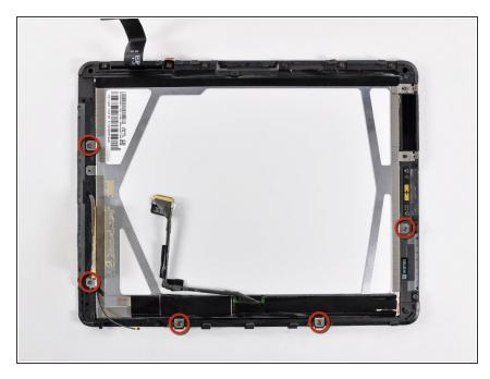
Remove the remaining T5 Torx screws securing the LCD to the black plastic display frame.
