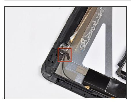
Remove the small strip of tape securing the antenna lead to the LCD.
