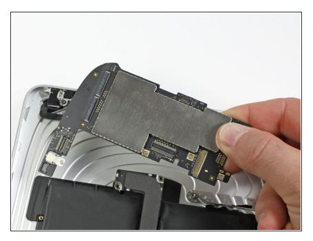
• Lift the logic board out of the rear panel assembly.
