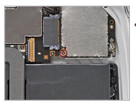
Remove the single T5 Torx screw securing the communications board to the rear case.
