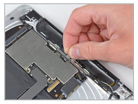
• Pull the GPS antenna ribbon cable out of its socket.
