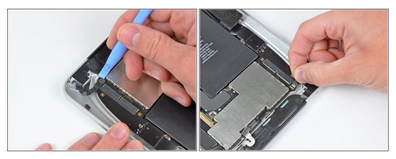
• Use the edge of an iPod opening tool to pry up the retaining flap on the headphone jack/microphone socket.
