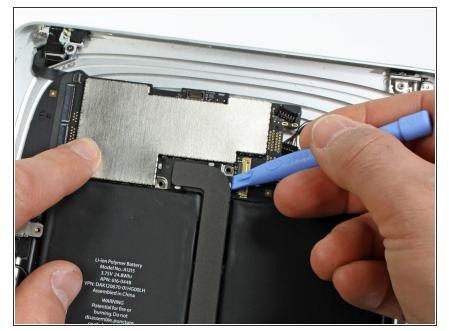
Use the edge of an iPod opening tool to carefully pry the dock cable connector straight up off the logic board.
