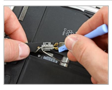
Pry the Wi-Fi and Bluetooth antennas up off their respective sockets on the Wi-Fi/Bluetooth board.
