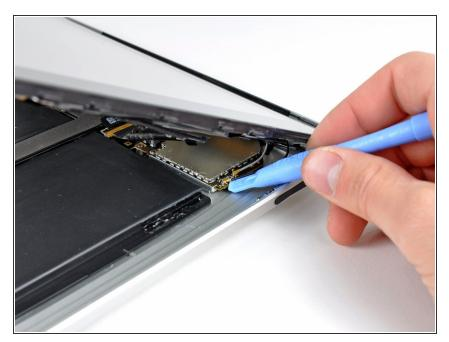
Use the flat end of a spudger to pry the antenna connector closest to the bottom of the iPad up off its socket on the communications board.
