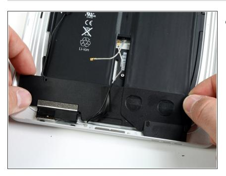
Lift the speaker assembly and push it forward until the ports clear the bottom side of the rear panel assembly.
