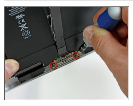
Remove the two 2.84 mm T5 Torx screws securing the dock connector cable to the rear panel assembly.
