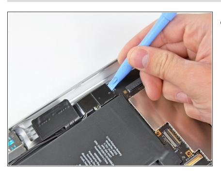
Use the edge of an iPod opening tool to pry the SIM board connector up off it socket on the logic board.
