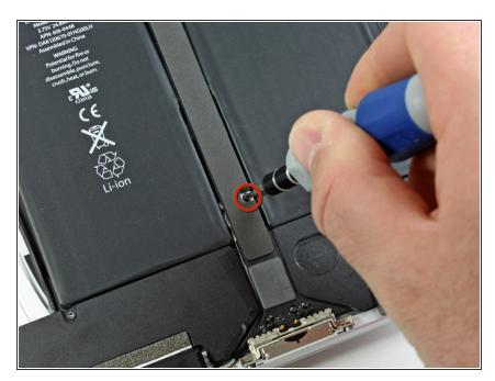
Remove the single 2.84 mm T5 Torx screw connecting the dock connector cable to the rear case assembly.
