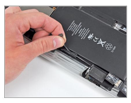
Deroute the speaker cable connector from under the black sticker attached to the left side of the rear panel assembly.
