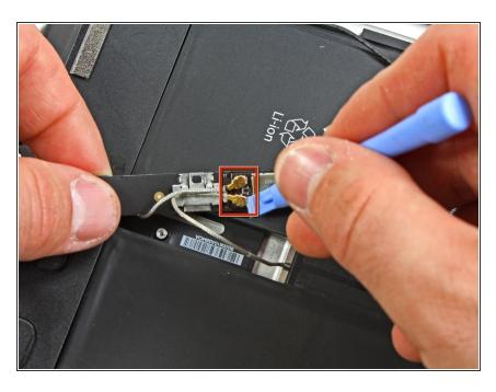
Carefully pry the Wi-Fi and Bluetooth antennas up from their respective sockets on the Wi-Fi/Bluetooth board.
