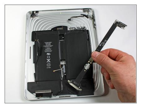
Lift the dock connector cable out of the rear panel assembly.
