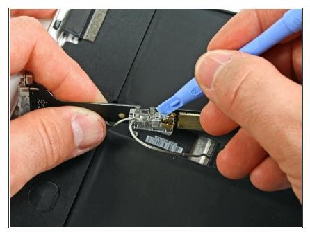
Using a plastic opening tool, carefully remove the plastic cover shielding the WiFi/Bluetooth board and dock connector cable.
