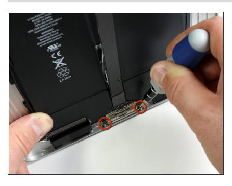
Remove the two 2.84 mm T5 Torx screws securing the dock connector cable to the rear case.
