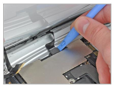
Use a plastic opening tool to remove the ambient light sensor connector from its socket by gently prying upward.
