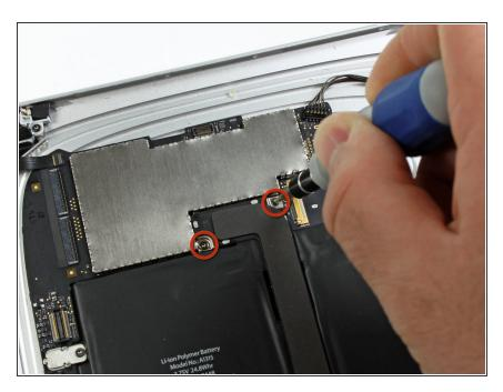
Remove the two 4.56 mm T5 Torx screws securing the dock connector cable to the main board.
