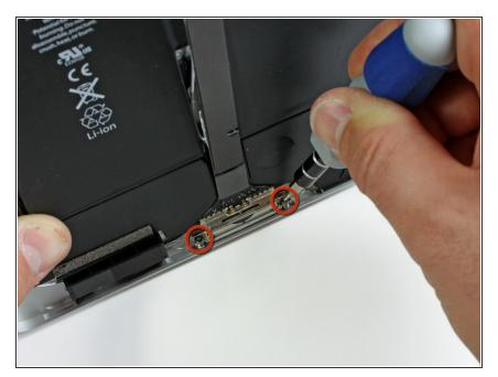
Remove the two 2.84 mm T5 Torx screws securing the dock connector cable to the rear panel assembly.
