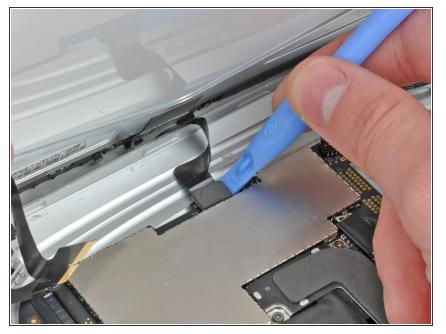
Use a plastic opening tool to remove the ambient light sensor connector from its socket by gently prying upward.
