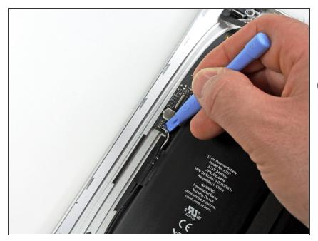
Use the edge of a plastic opening tool to disconnect the speaker connector from the logic board.
