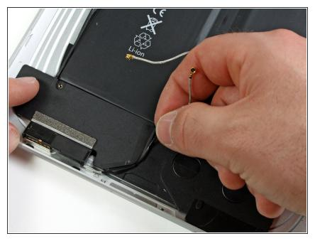
• De-route the Wi-Fi antenna through its channel in the speaker assembly.
