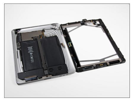
• Remove the display assembly from the rear panel assembly.
