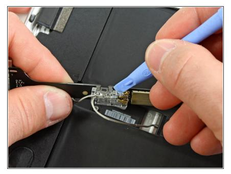
Carefully remove the plastic cover over the WiFi/Bluetooth board and dock connector cable using a plastic opening tool.
