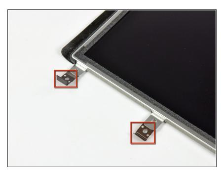
If they are still in good shape, transfer the clips and EMI tape near the bottom of the LCD to your new LCD.
