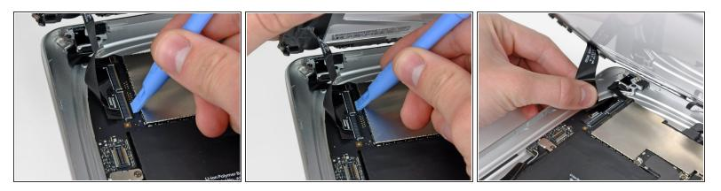
• Use the edge of a plastic opening tool to flip up the retaining flaps holding the digitizer ribbon cables in their sockets on the logic board.
