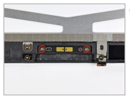
Remove the two T5 Torx screws securing the home button switch board to the display frame.
