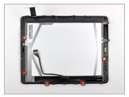
Remove the remaining T5 Torx screws securing the LCD to the black plastic display frame.
