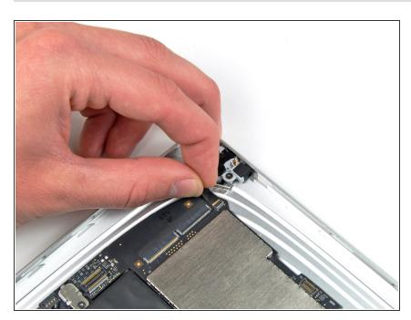
Carefully pull the headphone jack cable out of its socket on the logic board.
