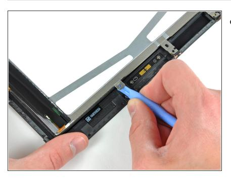
Repeat the process detailed on the previous step to pry up the display around the three sides opposite the digitizer cable side of the display.
