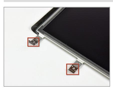
If they are still in good shape, transfer the clips and EMI tape near the bottom of the LCD to your new LCD.
