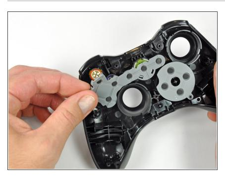
Remove the rubber pad from the back of the input buttons.
