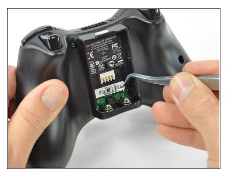
Use a pair of tweezers to peel the barcode sticker from the battery compartment.
