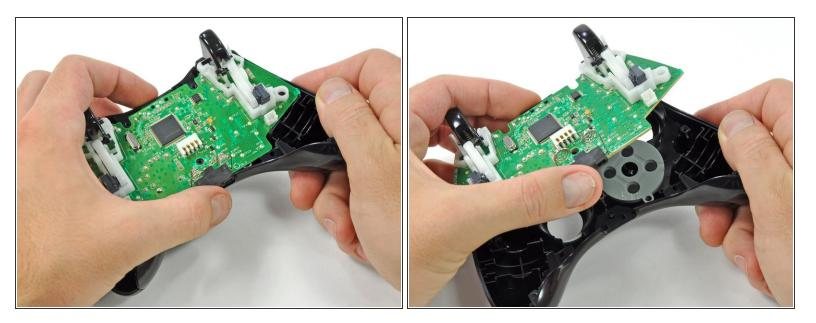
Lifting from the headphone jack and power plug, remove the logic board from the front case.
