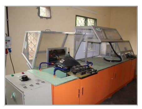
The CRT glass body can be separated into panel glass, funnel glass, shadow mask and phosphor coating (as shown in the picture on the right: CRT dismantling equipment at the WEEE Centre, Nairobi, Kenya).
