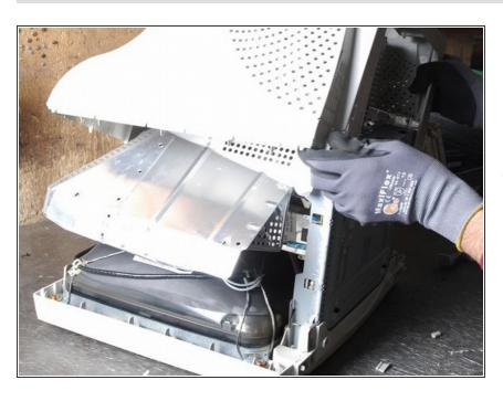
Remove the plastic casing by unscrewing all the screws in the cover (generally around 4). Clean the casing properly by removing all the foreign materials in the plastic such as labels, rubber mountains etc.
