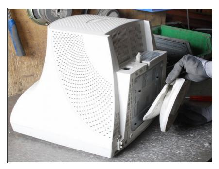
Before doing anything the monitor has to be placed face down to protect the monitor screen from breaking.
