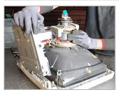
There are generally two Printed Wiring Boards (PWB) in a monitor. A small PWB is attached at the base of the monitor screen by glue or a screw. A bigger PWB is attached at the back. Particularly the bigger PWBs might need further dismantling.
