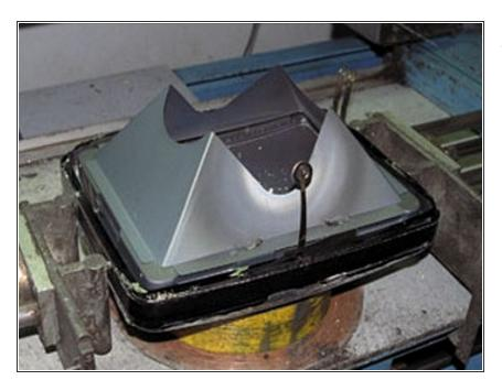
Remove the shadow mask and place it aside separately together with the ferrous metals.
