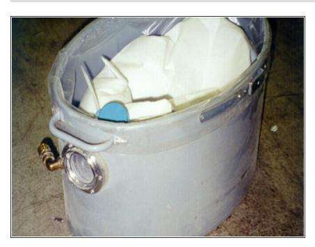
Store the phosphor layer or the vacuum cleaner bag containing it, respectively, separately in a bin with a cover.
