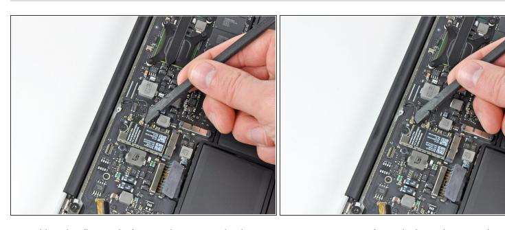
Use the flat end of a spudger to pry both antenna connectors up from their sockets on the AirPort/Bluetooth card.
