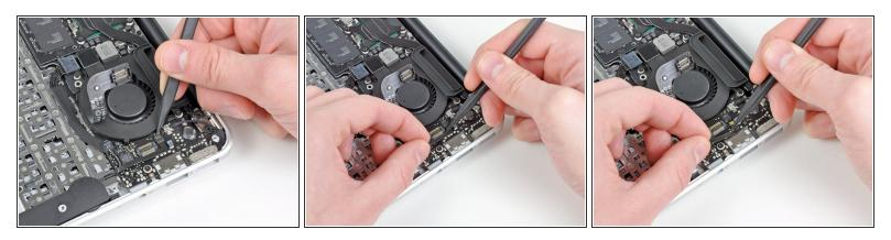
• Use the tip of a spudger to flip up the retaining flap on the microphone ribbon cable ZIF socket.
