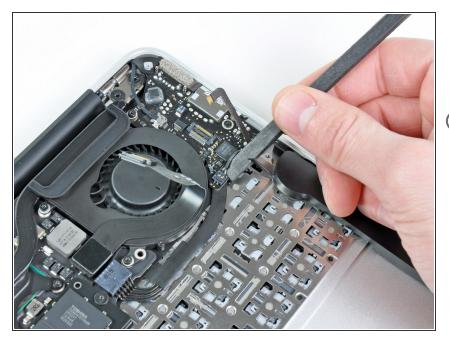
• Use the flat end of a spudger to pry the left speaker connector up and out of its socket on the I/O board.
