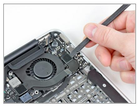
• Use the flat end of a spudger to pry the I/O board cable connector upward out of its socket on the I/O board.
