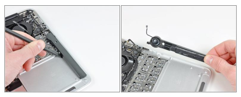
• Use the flat end of a spudger to pry the left speaker off the adhesive securing it to the upper case.
