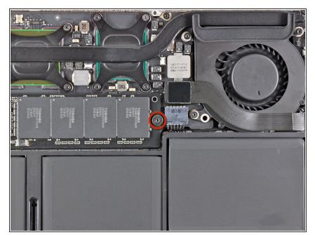
Remove the single 2.9 mm T5 Torx screw securing the SSD to the logic board.
