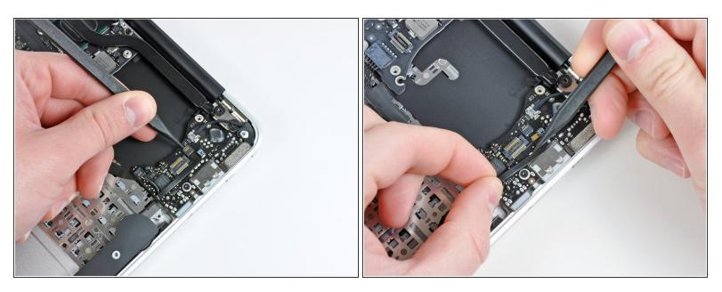
• Use the tip of a spudger to carefully flip up the retaining flap on the microphone cable ZIF socket.
