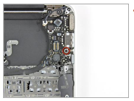
Remove the single 3.6 mm T5 Torx screw securing the I/O board to the upper case.
